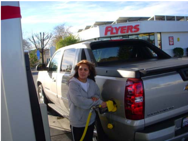
This guest saw the news and came over to fuel up at 85 cents per gallon. Her yellow gas cap hanging below the nozzle is one indicator of a Flex Fuel Vehicle.
